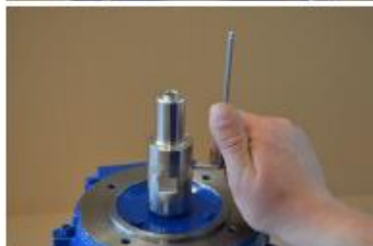
Fig 3.3.10 Loosen the lock screws [161] and remove the shaft extension [16].
