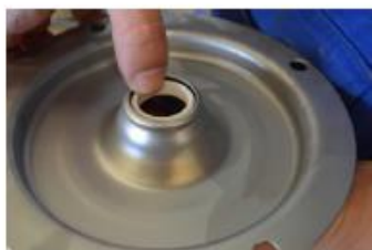
Fig 3.3.7 If necessary, push out the static part [15B] of the mechanical seal. NOTE! Apply some alcohol or water before pushing out of the mechanical seal.
