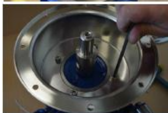
Fig 3.3.9 Remove the screws [121] and washers [122] holding the back cover [11] to the motor [10].
