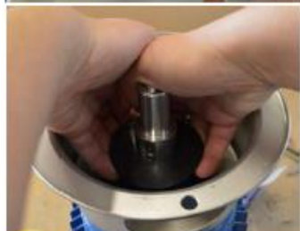
Fig 3.3.8 Remove the deflector [17].
